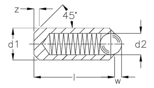
$\begin{array}{ll} \text{d1} & = 6.0 \\ \text{d2} & = 4.5 \\ \text{I} & = 15 \\ \text{Spring pressure N bottom} = 31.0 \\ \text{Spring pressure N top} & = 18.0 \\ \text{W} & = 1.50 \\ \text{z} & = 0.30 \\ \end{array}$
